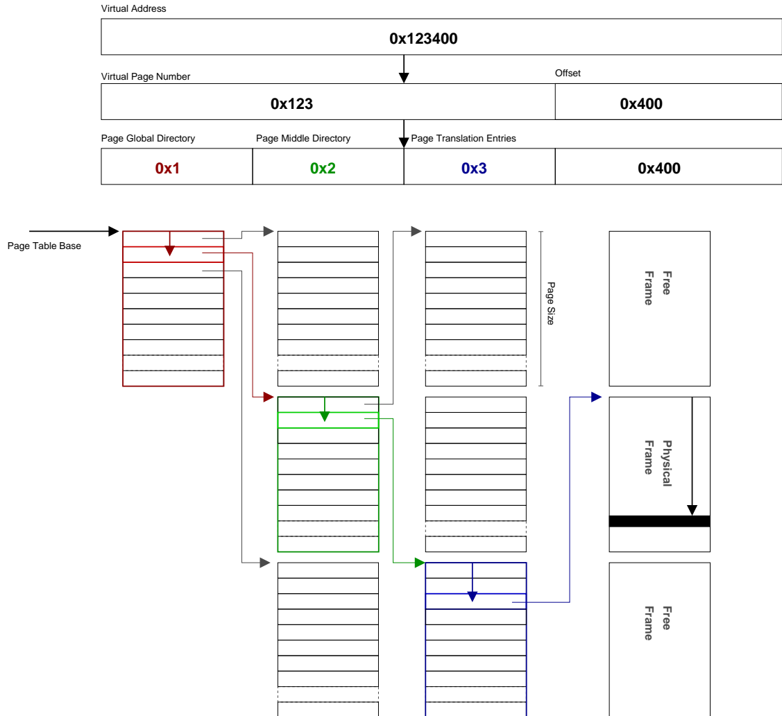
Figure 6.9. Illustration of a hierarchical page-table
